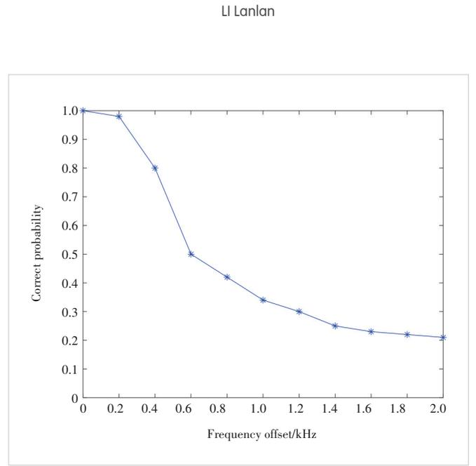
**Figure 7. Accuracy of synchronization under different frequency offsets**
