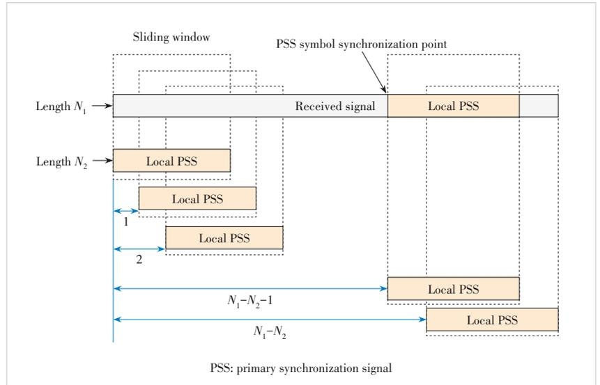
**Figure 1. Traditional PSS detection algorithm**
