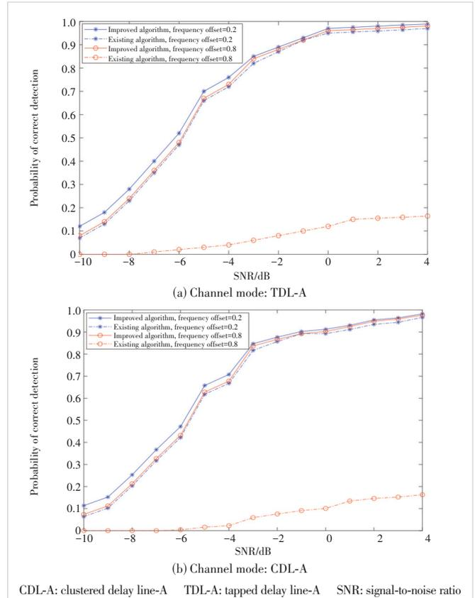
Figure 5. Probability of primary synchronization signal search algorithm
