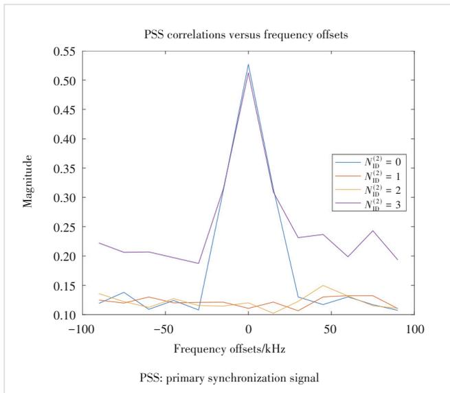
Figure 3. Correlation peaks of superimposed signals
