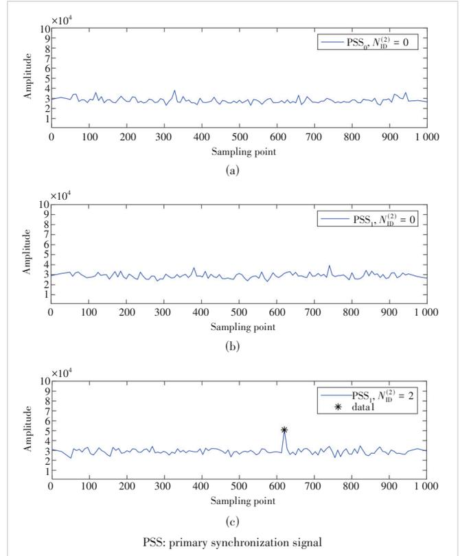
Figure 4. Correlation peak plot calculated by proposed algorithm
