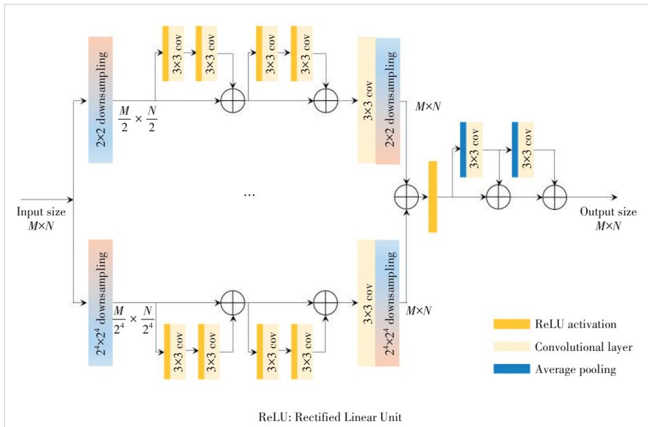
Figure 3. An elaborate schematic representation of model  $s_\theta$  utilizing the RefineNet architecture. This fundamental block is cascaded  $D$  times in sequence
