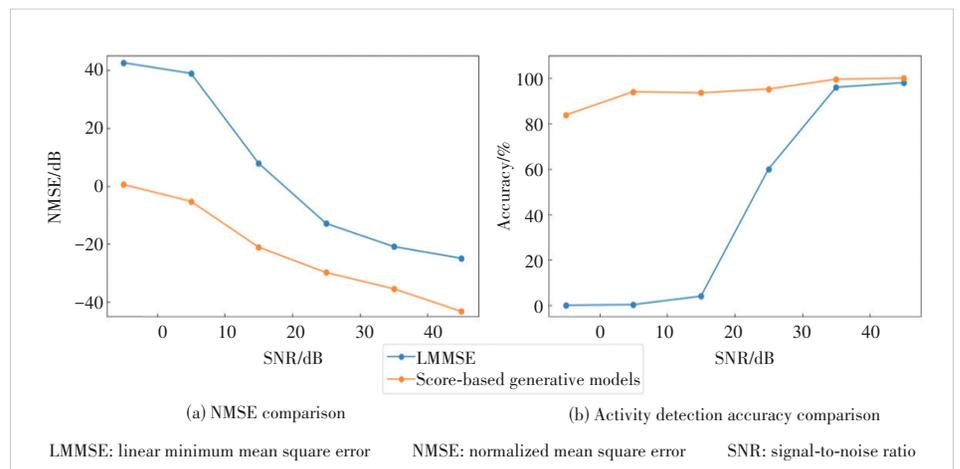
Figure 5. Performance comparison of channel estimation methods
