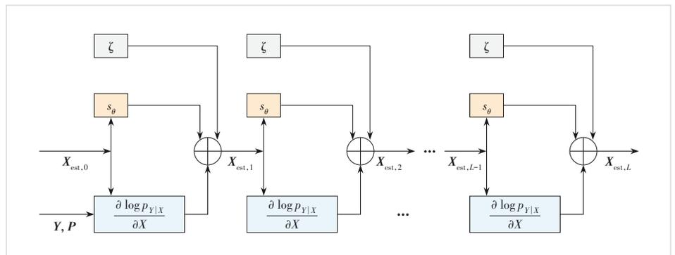
Figure 1. A step-by-step process for estimating  $X$  by employing a score-based model in conjunction with the known matrices  $Y$  and  $P$
